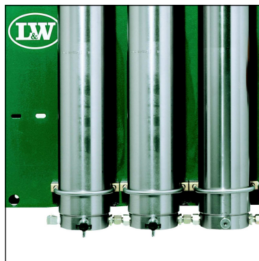
Fig. 3 - Loosen u-clamps and pipe connections
