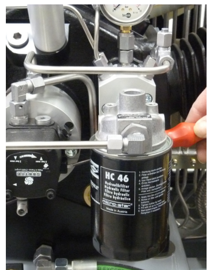
Adjusting the oil pressure
