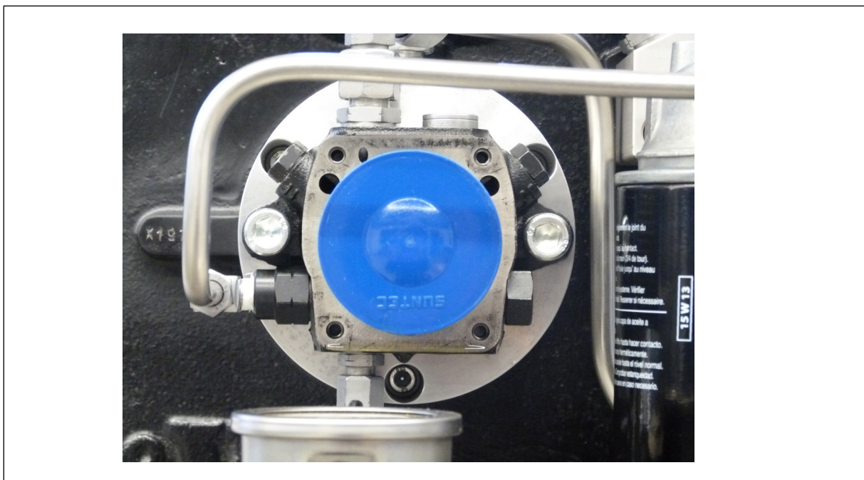
Correct oil sieve mounting direction
