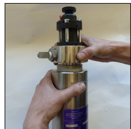
Fig. 3 - Open filter cover
