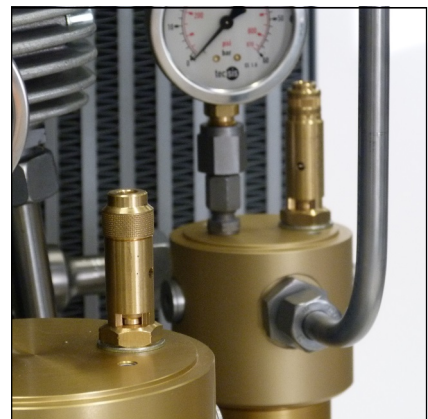
Safety valve 1st and 2nd stage
