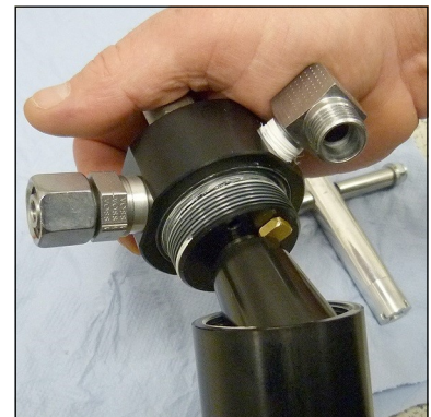
Fig. 3 - Turn off and remove separator head
