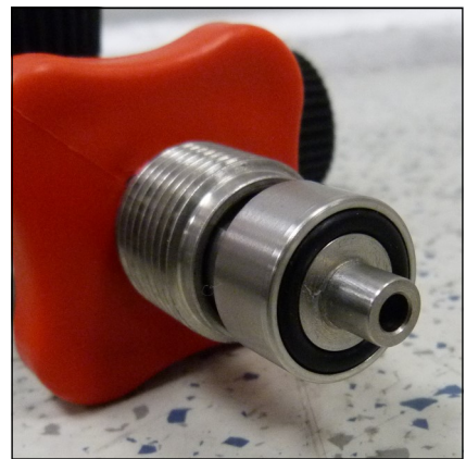
Fig. 1 - O-ring at the filling valve
