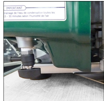
Fig. 1 - Condensate drain valve 1.stage
