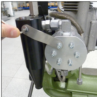
Fig. 1 - Loosen mounting screws
