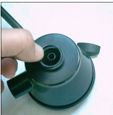
Fig. 4 - Place o-ring into the groove
