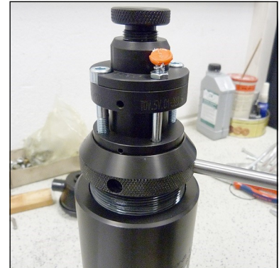
Fig. 1 - Remove/screw in filter cover
