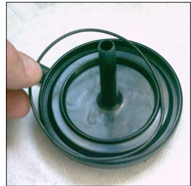
Fig. 3 - Place o-ring into the filter housing
