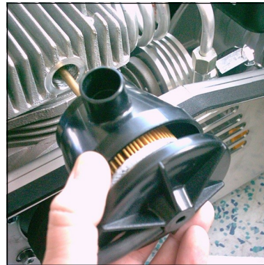
Fig. 2 - Pull out filter housing carefully
