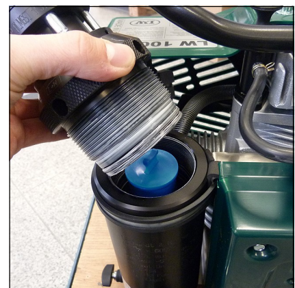
Fig. 2 - Remove filter housing cover
