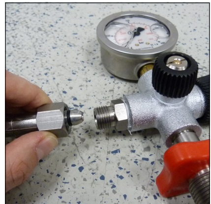
Fig. 2 - O-ring at the filling hose
