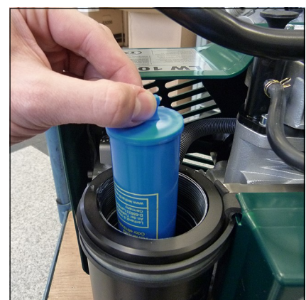
Fig. 3 - Pull out the filter cartridge by the catch and insert a new cartridge
