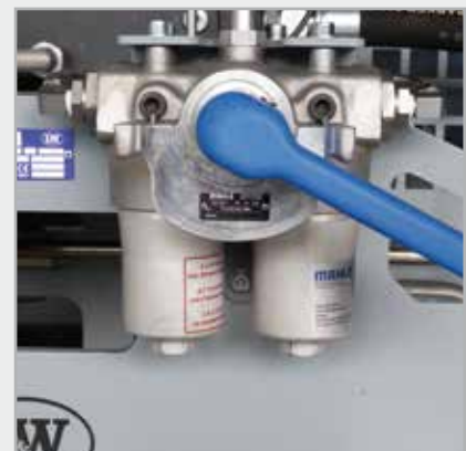
Changeable oil distribution for an oil change during a running machine (option)
