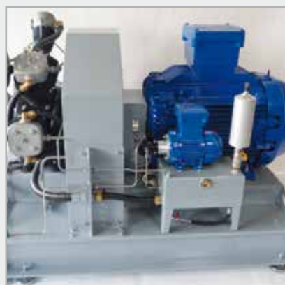
LW1300 EG with additional oil lubrication circuit
